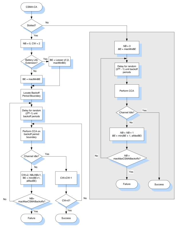
Figure 5: The Unslotted CSMA-CA Algorithm
