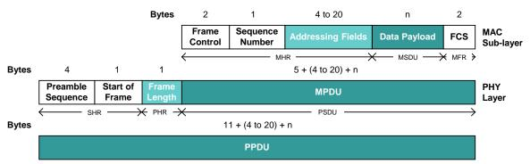
Figure 1: Schematic View of Data Frame
