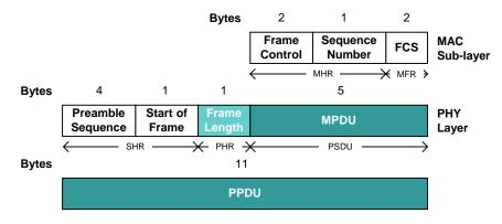
Figure 3: Schematic View of Acknowledgement Frame
