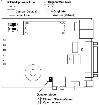
**Note:** The Speaker Mode jumper is for a modem with the voice option
