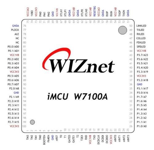
Fig 1. W7100A 100pin LQFP package
