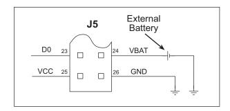
Figure C-1. External Battery Connections at Header J5
