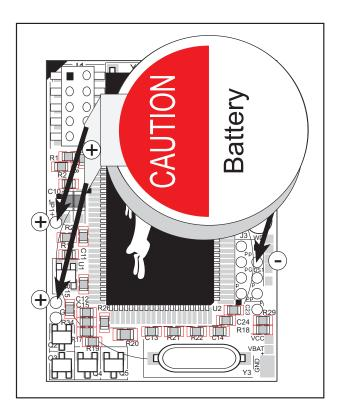
Figure C-2. Installing Onboard Backup Battery on RCM2300
