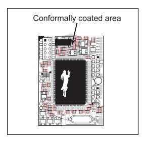
Figure A-5. RCM2300 Areas Receiving Conformal Coating
