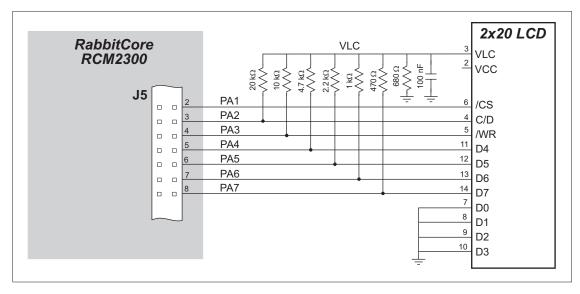
Figure E-3. Sample LCD Connections
