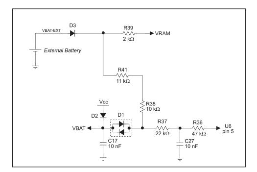
Figure C-4. RCM2300 Battery-Backup Circuit
