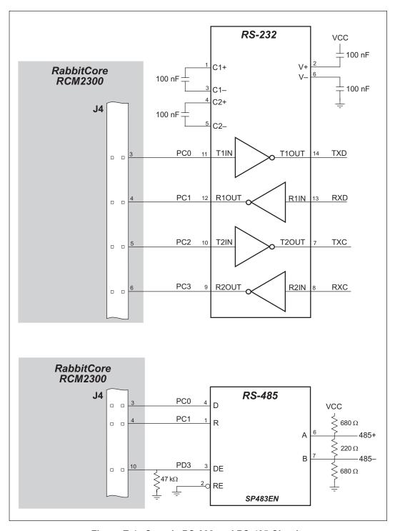
Figure E-1. Sample RS-232 and RS-485 Circuits
