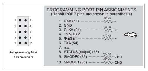
Figure D-1. Programming Port Pin Assignments
