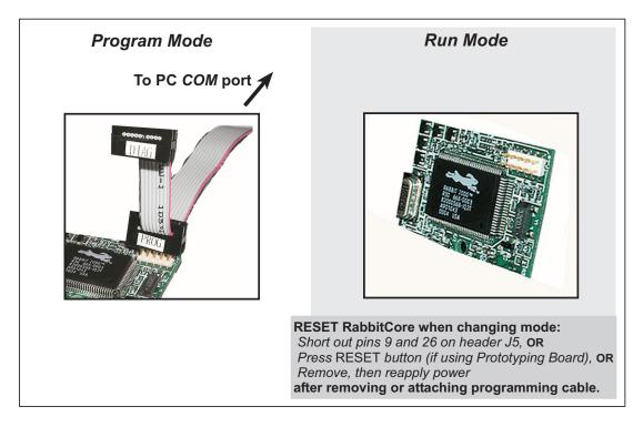
Figure 3. Switching Between Program Mode and Run Mode
