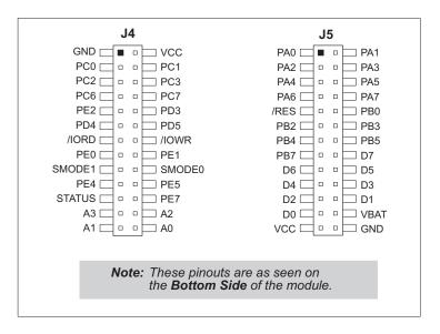
Figure 2. RCM2300 I/O Pinout
