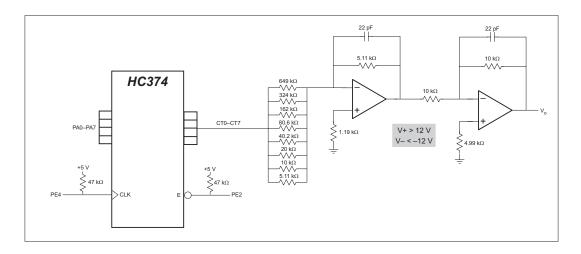
Figure E-5. Sample D/A Converter Connections
