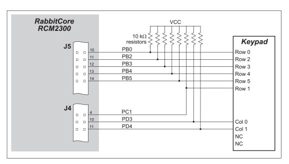
Figure E-2. Sample Keypad Connections
