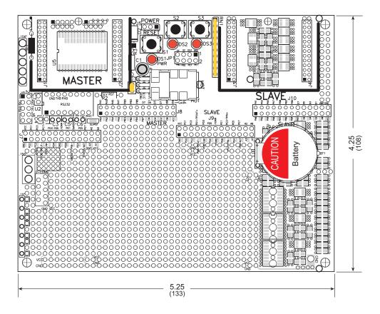
Figure B-1. RCM2300 Prototyping Board Dimensions
