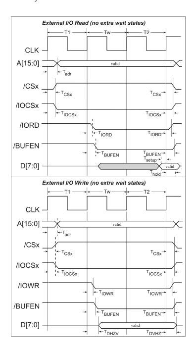
Figure A-4. Memory Read and Write Cycles
