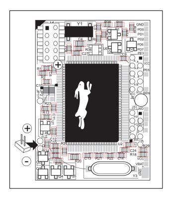
Figure C-3. Installing Optional Battery Connector on RCM2300
