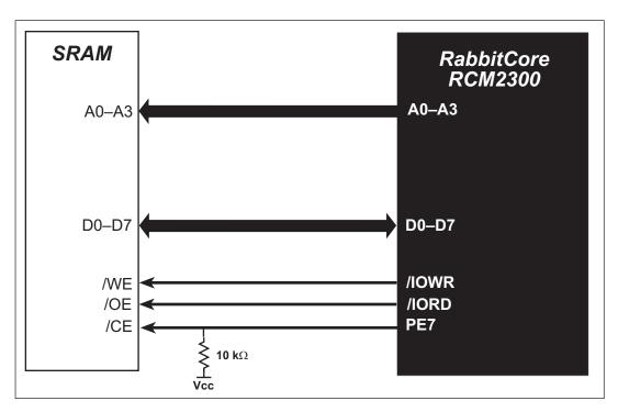
Figure E-4. Sample External Memory Connections
