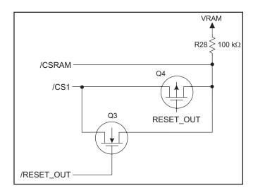
Figure C-5. Chip Select Control Switch
