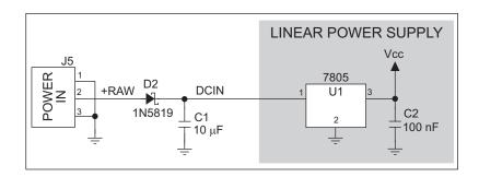
Figure B-2. Prototyping Board Power Supply
