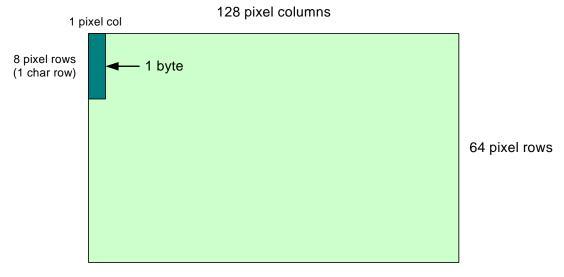
Figure 1: Data Display on LCD Screen
